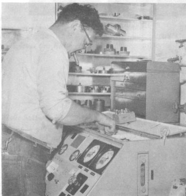
MM1 J.B. SMITH Testing flow control valves on type II test stand.
