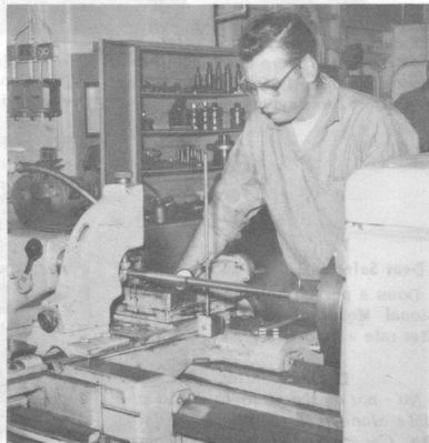
MR3 JADIN Turning an outboard motor shaft for EOD
