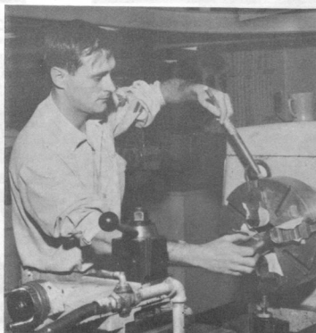
MR2 M.A. DEMARCO Setting up to make a spud for a steady rest
