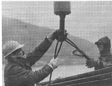
SA Lynch and SN Dameron fasten a crane hook to a cable in preparing to lift cargo with one of the ship's travelling cranes.
