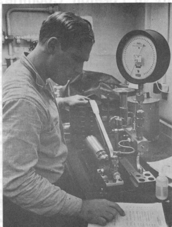
IMSN L. Austin tests pressure gauges with dead weights.
