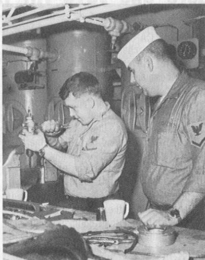
Crews, BT3, is observing Young, BT2, repairing a steam regulator, a vital part of the Fuel Oil service Pump.
