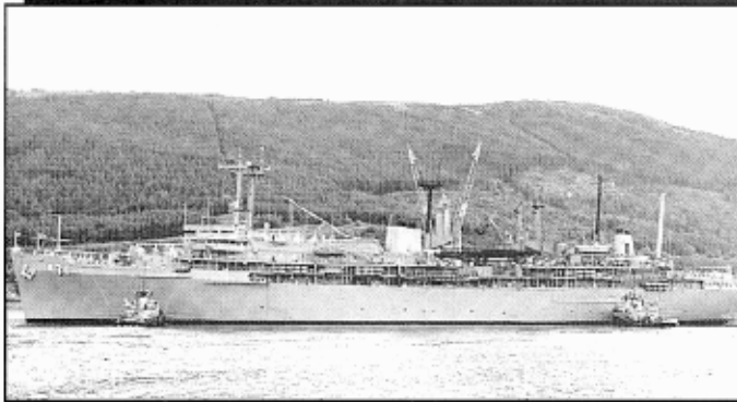
Largest in displacement was the 20,500-ton submarine tender USS Hunley (AS-31) built at Newport News in 1961 and modified in 1973/1974 to support the Poseidon missile program. Sistership Holland (AS-32) was built by Ingalls a year later. This 1962 photo shows Hunley as built with a large gantry crane for missile loading located well aft. Inset photo shows the much-altered Hunley at Holy Loch circa 1990 being pushed into her mooring by the harbor tugs Piqua and Natick .
